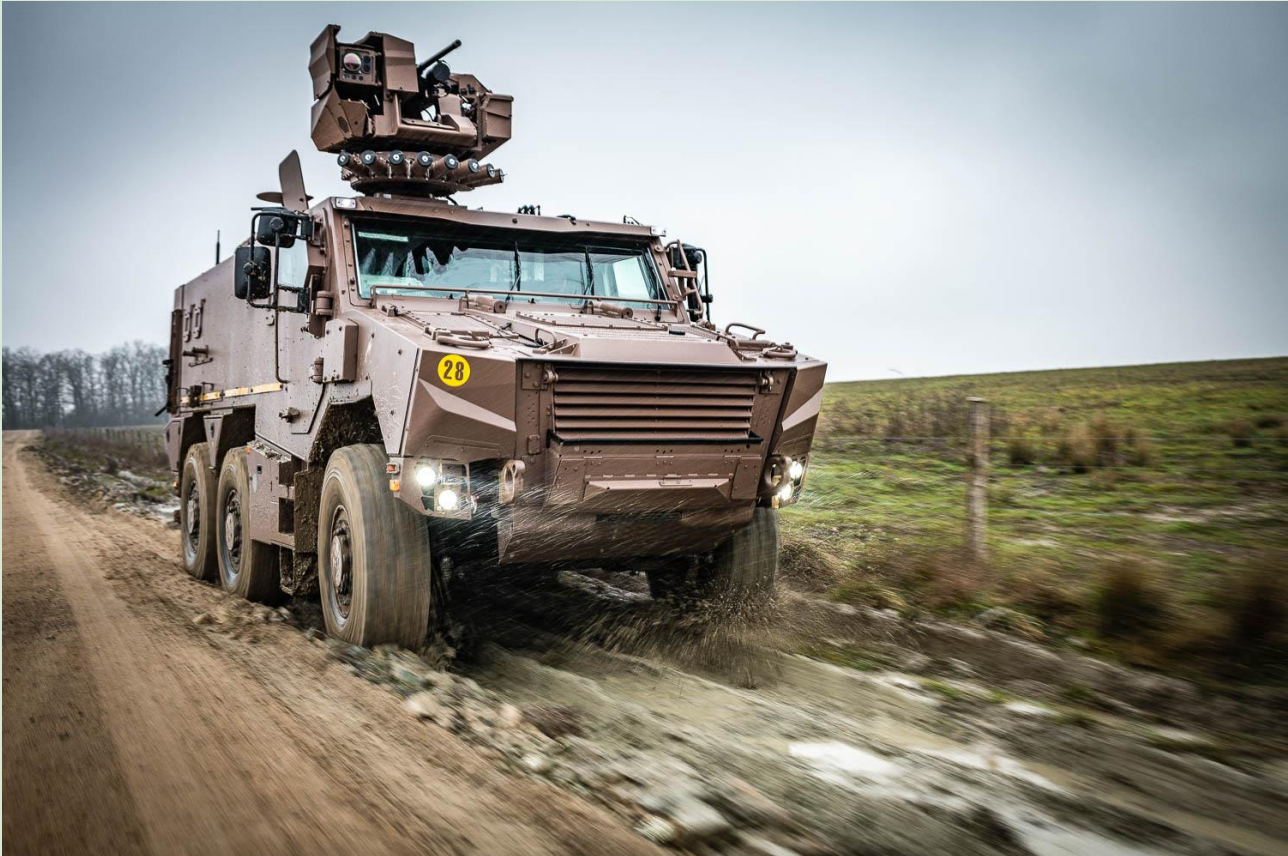
A French Army Griffon equipped with a Hornet RCWS Credits: Arquus
