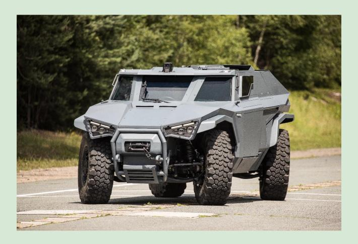
The Scarabee was presented publicly for the first time in its all-electric mode in October 2020 during the Arquus Days in Satory, France. Thanks to its 70kW hybrid engine, the Scarabee offers the stealthiest acoustic footprint on the market when in 100% electric mode. Its high-capacity (12kWh) li-ion batteries enable the Scarabee to travel the last kilometers to target silently and get as close as needed to the enemy without getting detected, both for reconnaissance and attack purposes.
