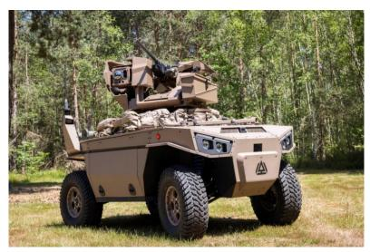
Equipped with a hybrid electric/diesel propulsion system ensuring discreet mobility, the DRAILER is a robot with proven technologies, offering autonomy suitable for operational theaters. This versatile robot is a valuable companion in the field! It can operate with a payload of up to 700 kg, while possessing off-road capabilities meeting high-intensity expectations.
